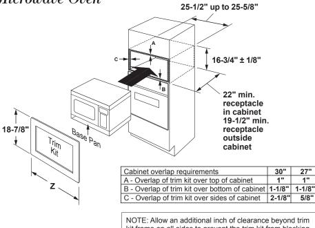
kit frame on all sides to prevent the trim kit from blocking any outside adjoining cabinets/obstructions. Reference below drawing.
